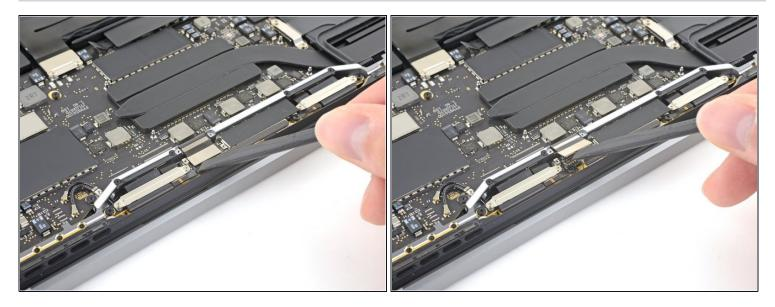
• Pry the display board flex cable straight up from its socket to disconnect it from the display board.
