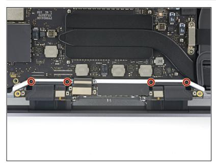
Remove the four 4.1 mm T3 Torx screws securing the spring hinges of the two display cables.
