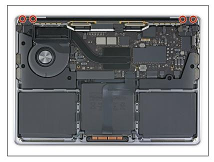
Remove the four 3.3 mm T3 Torx screws securing the plastic covers on top of the display hinges.
