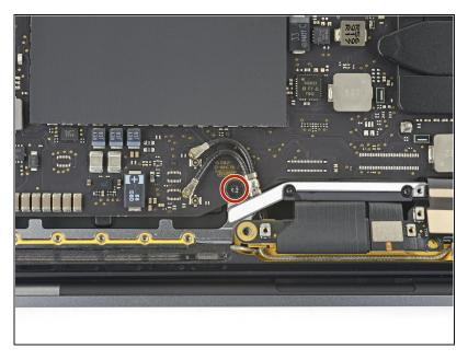
• Remove the 3.7 mm T5 Torx screw securing the two antenna coax cables to the main board.
