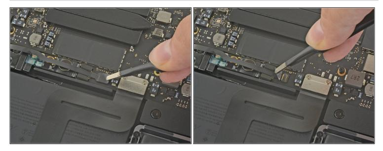
Gently peel back the small piece of tape covering the battery board data cable connector.
