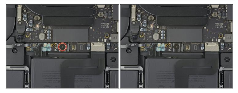
Use a T5 Torx driver to remove the 3.7 mm pancake screw securing the battery power connector.
