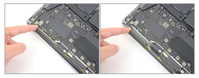
• Carefully remove the antenna assembly while simultaneously feeding the antenna cable bundle out from underneath the heat pipe.
