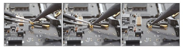
To reconnect each antenna cable, use tweezers to align the connector directly over its socket, and then press down with a spudger so it snaps into place.
