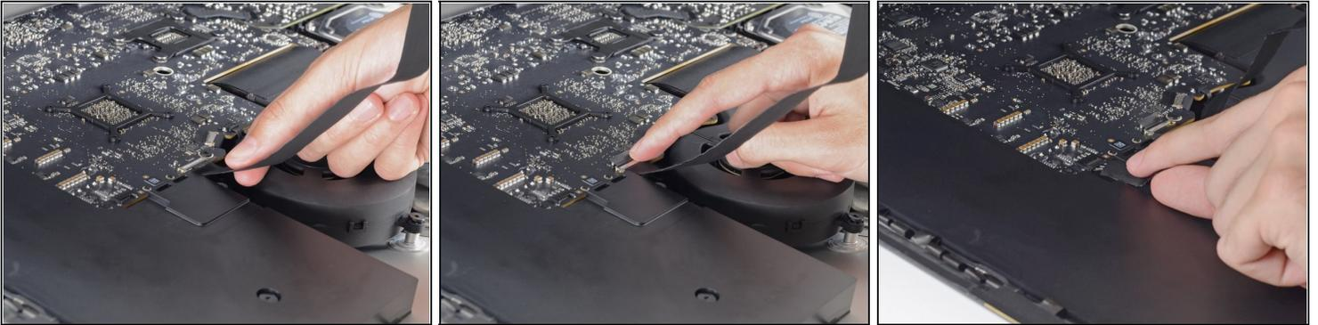
ⓘ *At this point it's a good idea to test your repair, in order to make sure your iMac works properly before you seal it back up. Follow the next three steps to temporarily reconnect the display cables and boot up your iMac prior to pulling the protective film off the adhesive strips.*
