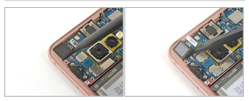
Use the point of a spudger to pry the front facing camera out of its recess.
