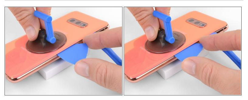
Insert an opening pick into the edge next to the opening tool. Leave the pick here to prevent the separated glue from re-adhering.
