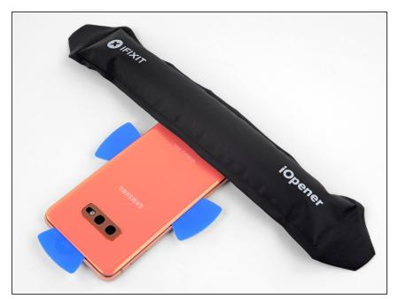
Apply a heated iOpener to the bottom edge of the phone for two minutes.
