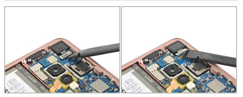
Use a spudger to pry up and disconnect the front facing camera connector from its motherboard socket.
