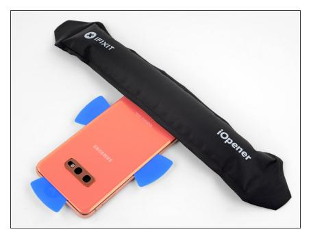
Apply a heated iOpener to the bottom edge of the phone for two minutes.
