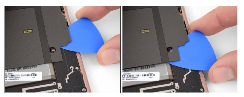
Slide an opening pick under the bottom right corner of the upper midframe to separate the adhesive holding it to the lower midframe.
