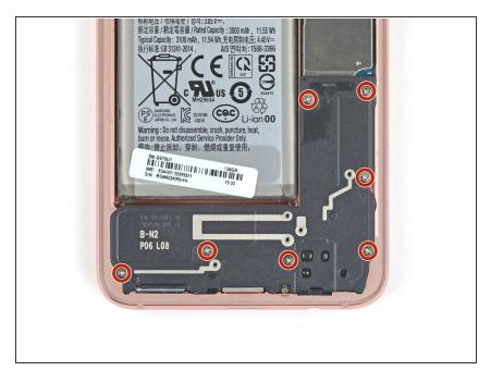
Use a Phillips driver to remove the seven 3.9 mm screws securing the loudspeaker.
