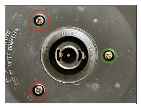
Remove the two Phillips screws (circled in red on the picture) and use a triangular bit to remove the third screw (circled in green on the picture)
