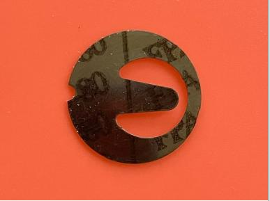
• I couldn't find just the bimetallic switch, so I purchased instead a replacement temperature control terminal for another type of Kettle on Amazon. The strip appeared to be pretty standard and slides right out when you lift it from the bottom notch.
