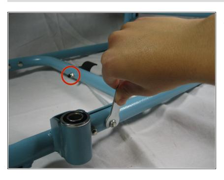
Remove the bolt with the rubber cap that attaches the air pump to the center support on the bottom.
