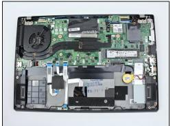
• Lift the battery near the connector and remove it from the system.
