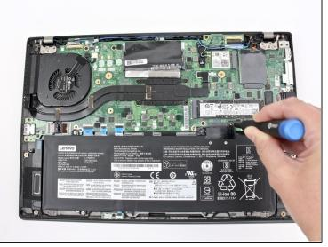
• Use the Phillips #1 screwdriver to remove four 4.5mm screws that hold the battery down to the mid frame.
