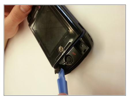
On the front of the device, pry off the top right, top left, bottom right, and bottom left buttons
