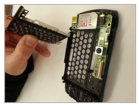
Using the appropriate size Phillips screwdriver, remove any screws that are attached or associated with the keypad and carefully remove keypad from the device.
