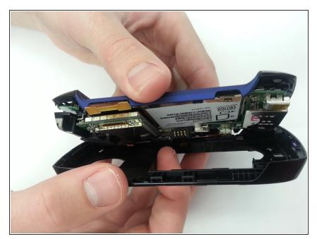
Once screws are dismantled, use plastic opening tool to assist separation of the top half of device from the bottom half
