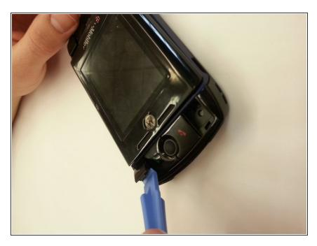
• When looking at the front of the phone, use the Plastic Opening Tool to pry off the four buttons located in each of the corners on the front.
