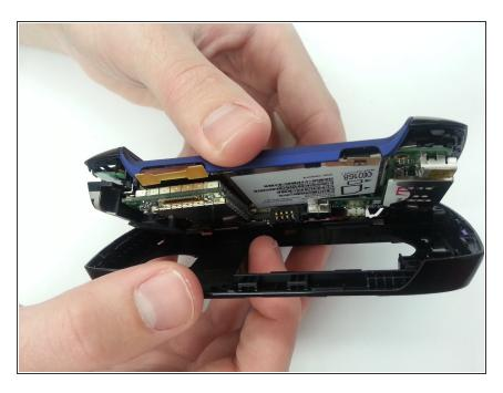
After removal of the back screws, use the Plastic Opening Tool to carefully separate the top and bottom halves of the device.
