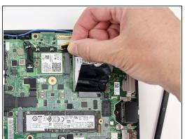
Use the spudger to disconnect the LCD cable from the motherboard.
