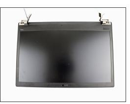
Carefully rotate the hinges upward and remove the bottom of the machine from the LCD unit.
