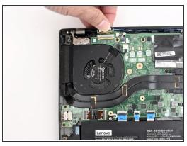
Disconnect the camera cable from the motherboard using a spudger.
