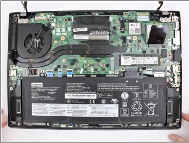
Remove all antenna cables from their routing.
