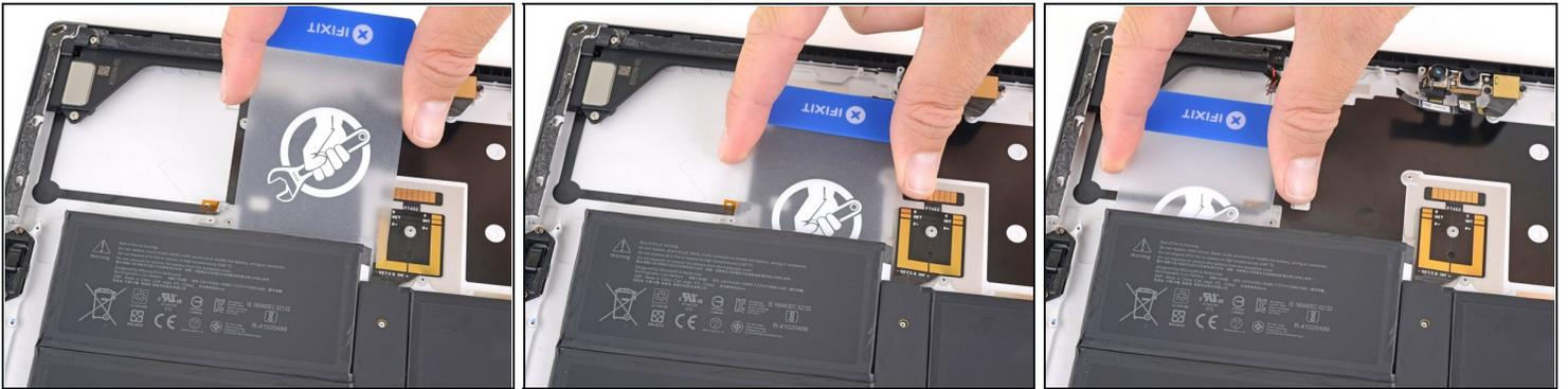
**⚠ Take care not to puncture or bend the battery with your tools—a punctured or bent battery may leak dangerous chemicals or cause a thermal event.**
