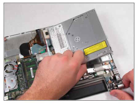
• Flip the CD Drive over carefully, lifting the right side and turning the drive in order to reveal the attachment.
