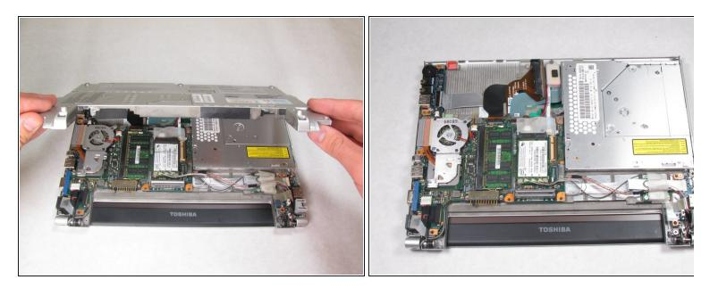
• Pull up on the back casing and remove it, revealing the CD drive.
