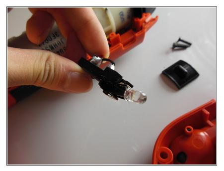
• Pull the black plastic piece up out of the slot in the drill body that it fits into.
