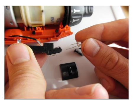
• Take your new LED and slide it back into the plastic housing in the same orientation as the old LED.
