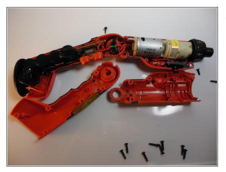
• Lift one side of the drill casing off of the drill. Note that the drill casing consists of two pieces on either side of the drill.
