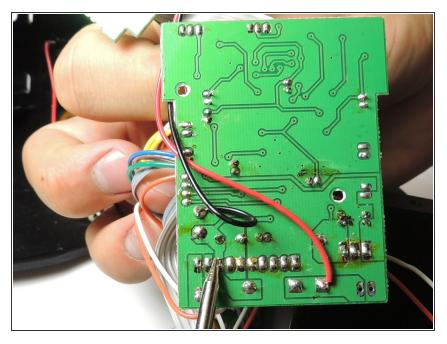
• Solder each wire to corresponding input on the motherboard.
