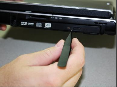
Using the tweezers, insert them into the small hole next to the CD drive button.
