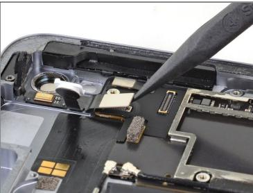
• Use the pointed end of a spudger to disconnect the power button assembly's press connector from its socket.
