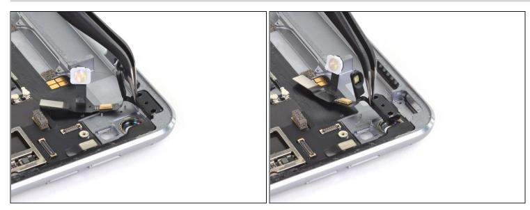
• Use a pair of tweezers to remove the power button bracket.
