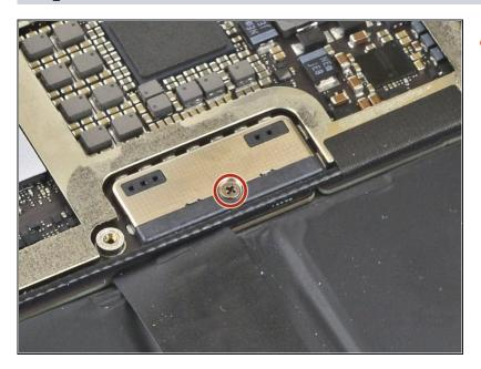
Use a Phillips driver to remove the 1.7 mm-long screw securing the battery connector.
