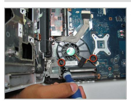
Remove the two 6mm screws with a Phillips #00 screwdriver.
