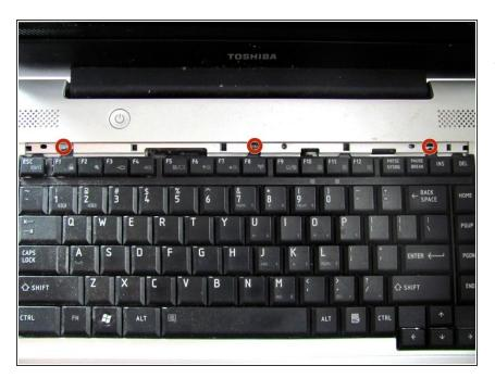
Remove the three 3mm screws with a Phillips#00 Screwdriver.
