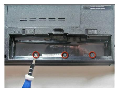
Remove the three 4mm screws with a Phillips #00 screwdriver.
