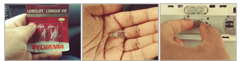
Replace the dead or broken bulb with a new bulb and insert it into the socket.
