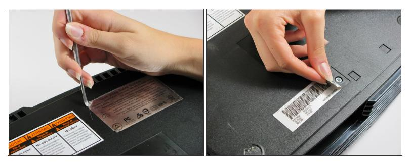
$\blacksquare$  There are 2 more screws hidden under the two labels on the bottom of the case.
