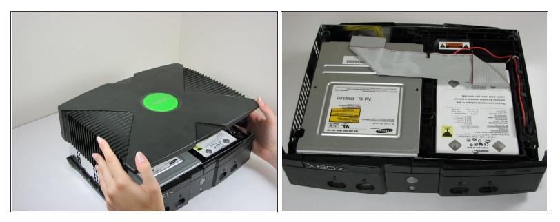
Once the bottom and top shells are no longer attached, carefully turn the Xbox right-side-up, lift and remove the top cover.
