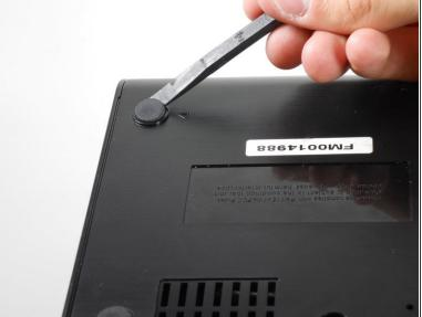
Slide a spudger under the two front rubber pads to expose two hidden screws.
