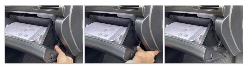
Push the lever connected to the right side of the glove box.
