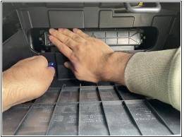
Place the filter cover and ensure both hinges click into the holder.
