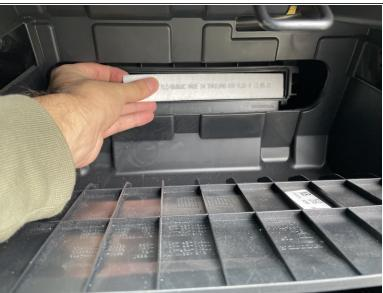
• Insert the new cabin filter with the direction indicated from the previous filter (downwards).
