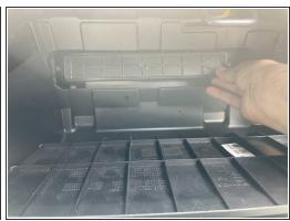
Push the left and right hinges to release the cabin filter cover.
