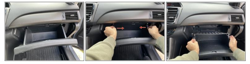
Push inwards on both sides of the glove box to release it.
