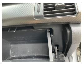
Insert the glovebox back into the dashboard and lock the tabs into place.
