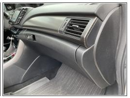
Pull the lever back onto the glove box hinge.
