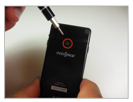
Remove the 3mm Phillips #00 screw on the back of the Insignia NS-4v17.
