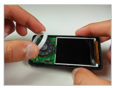
Remove the white plastic ring from around the scroll wheel using your fingers.
