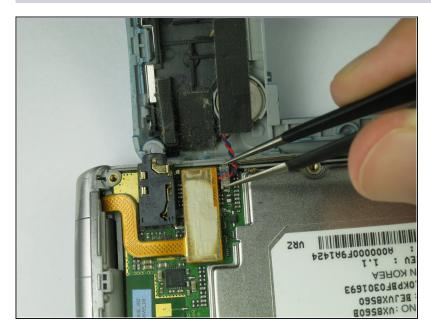
• Use tweezers to pull the clear end of the red and blue speaker cables away from motherboard.
