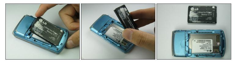
• Using your index finger lift and remove the battery from the phone.
