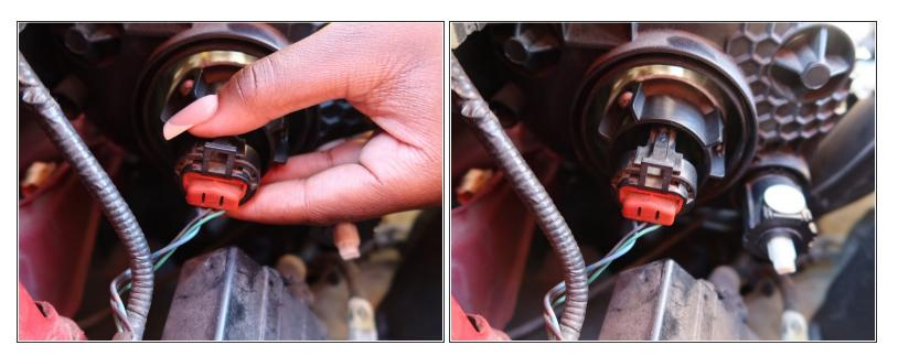
• Insert the connector into the bulb.
