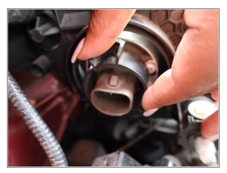
• Twist the plastic ring out from the bulb.
