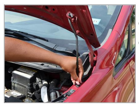
• Insert the support rod into the slot.
