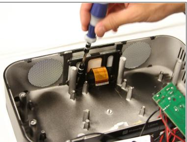
• Unscrew two 10mm silver screws at the base of the LCD screen to free it from the chassis.
