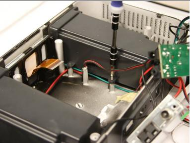
Unscrew four 7mm Phillips screws from the base of each speaker unit.
