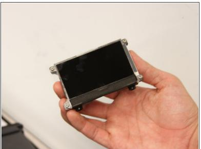
Gently pull up on the LCD screen to remove it.
