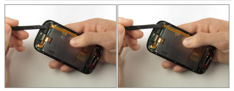
• Pry off the flex cable located at the top right of the display assembly using the flat end of a spudger.
