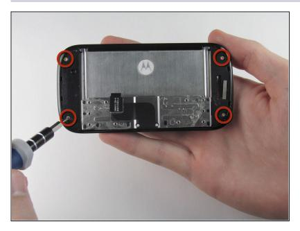
• Remove the four 3.0 mm T4 Torx screws at the corners of the phone.
