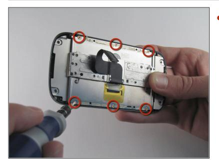
• Remove the six 3.0 mm T4 Torx screws that align on the phone's sides.
