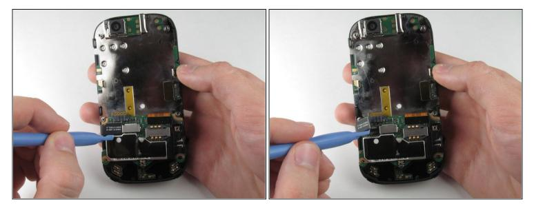
• Wedge the plastic opening tool underneath the black display connector and pry it off its socket on the motherboard.
