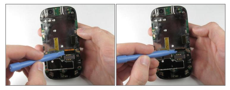
• Pry the orange keyboard connector from its socket on the motherboard using the edge of the plastic opening tool.
