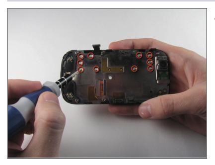
• Remove the ten 3.0 mm T4 Torx screws near the black display cable.
