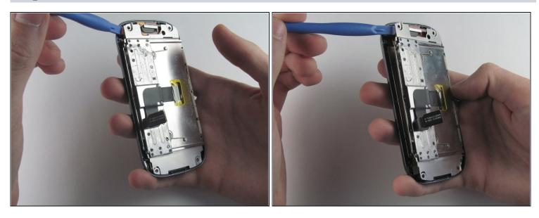
• Insert a plastic opening tool between the LCD shield plate and a corner of the keyboard slider plate.
