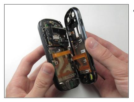
• Carefully separate the back casing from the rest of the phone.
