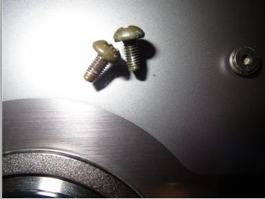
Remove the two screws on the top of the back cover. The second photo shows these 2 screws which have a fine thread and screw into metal.
