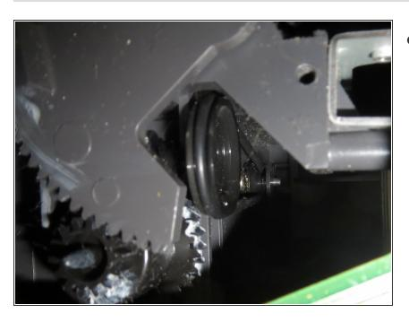
The new "O" Ring belt is fitted snugly and working.
