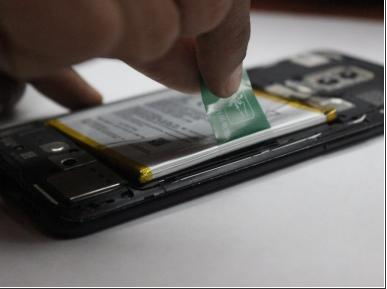
• Grip the green tab connected to the battery and pull the battery directly up and out.
