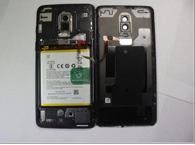
Gently lift up the back panel, with care not to damage the fingerprint sensor ribbon cable.
