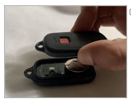
Reassemble the fob, using your hands to press the two parts together.
