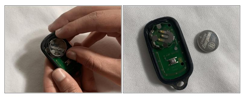
• Remove the battery from the fob by releasing it from the holder using a spudger or by hand.
