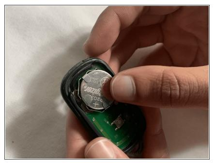
Insert the new battery by pushing it down.
