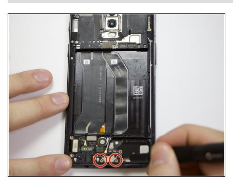
Using a Phillips #00 screwdriver, remove the two 2.3 mm screws with the screwdriver located on the two ends of the charging port.
