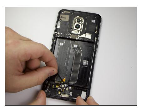
Pull the rubber strip up with your finger located just inside of the battery housing.
