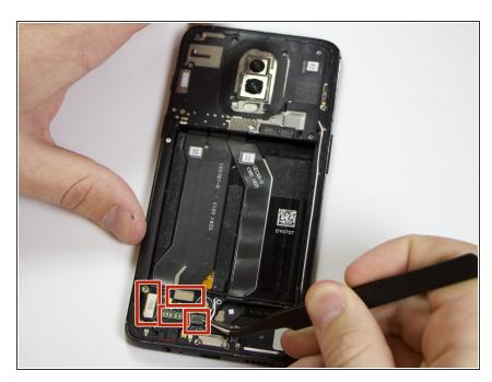
Gently disconnect the four connectors surrounding the charging port using a pair of tweezers.
