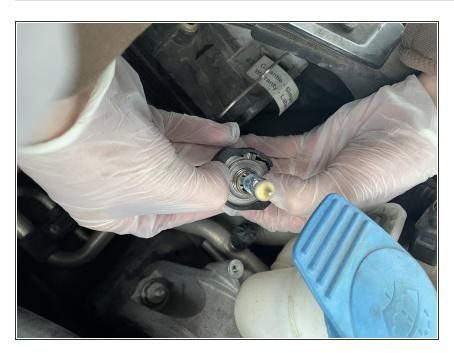
Insert the new halogen bulb into the casing.
