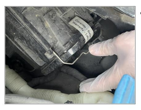
Close retainer clip by pushing down towards the bottom of the car to secure.
