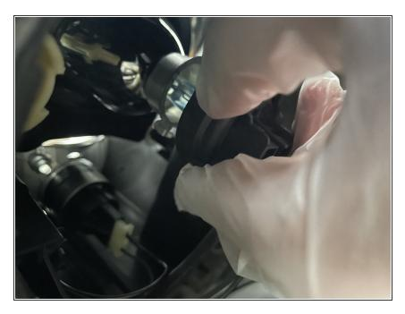
Insert bulb casing back into the socket.
