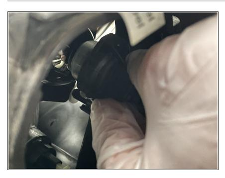
Unscrew the bulb casing.
