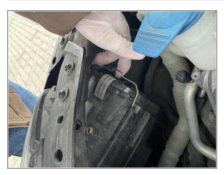
Pull up the retainer clip, pushing up towards the front of the car.
