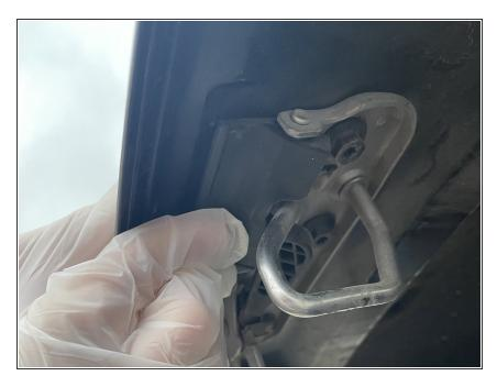
Pull the lever up to unlatch the hood.
