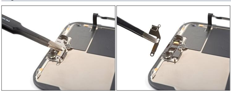
Use tweezers, or your fingers, to remove the front sensor assembly bracket.
