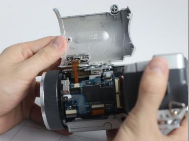
Remove the housing over the lens circuit board.
