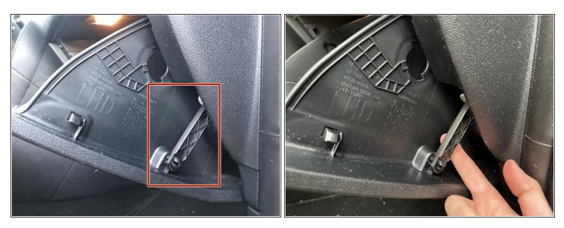
Carefully disconnect the latch on the right side of the glove box by pulling the latch away from the main glove box.
