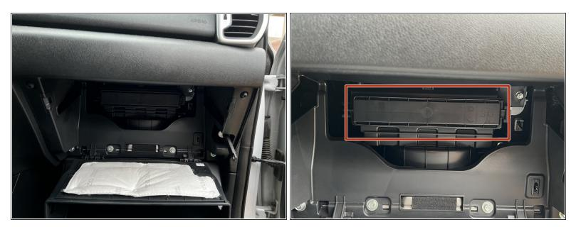
• Locate the rectangular air filter compartment directly behind the glove box.
