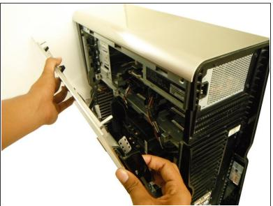
Remove the cover panel on the side of the computer by pulling out the latch on the back panel and pulling the panel downwards towards the ground.
