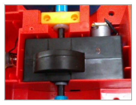
6v electric motor with capacitor for noise and spark suppressor wired across the terminals
