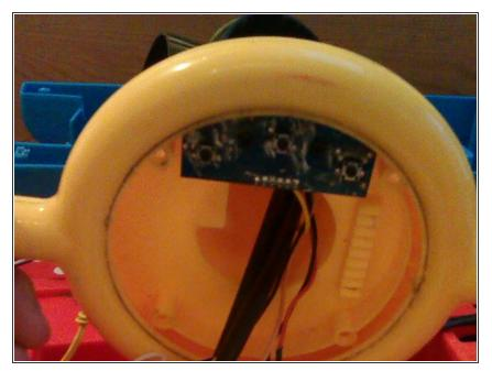
Has three switches to activate the music and connectors leading off to the motor, speaker, LED and battery
