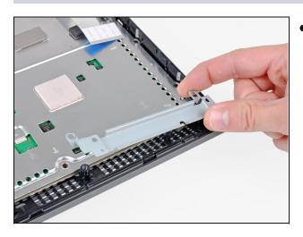
Remove the control board bracket.
