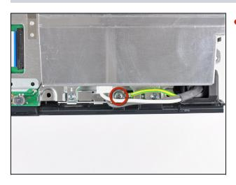
Remove the 7.7 mm Phillips screw securing the ground strap to the chassis.
