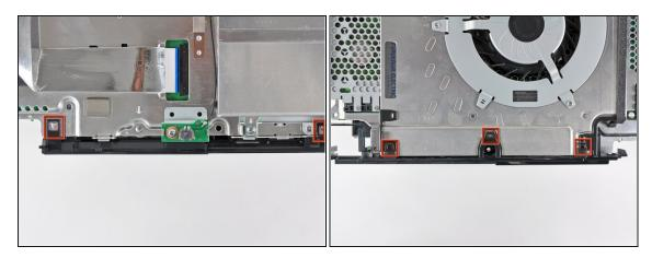
• While lightly pulling the rear cover away from the logic board assembly, use the flat end of a spudger to release the clips along the top and bottom edges of the rear cover.
