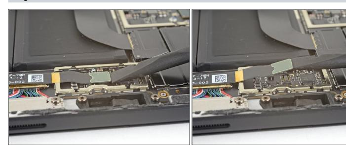
• Use the flat end of a spudger to pry the microSD card reader connector up and out of its socket on the motherboard.
