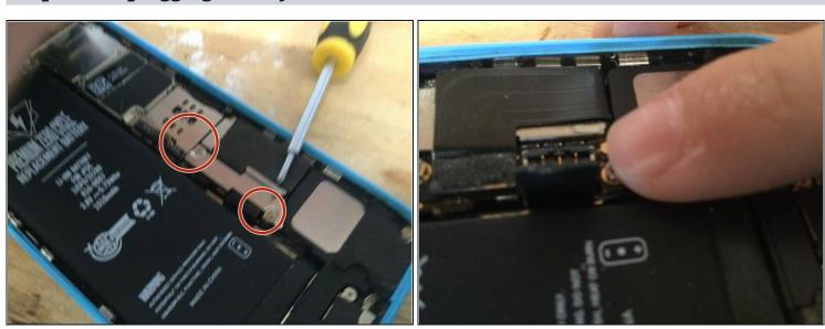
Unplug battery take out Phillips head screws on the cover and unplug the battery.
