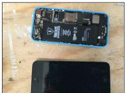
• Take off screen cables by removing the shield with four Phillips head screws
