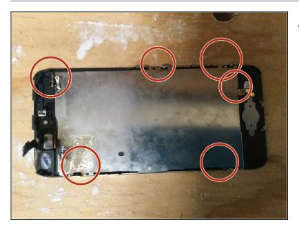
Remove back plate with six Phillips head screws.
