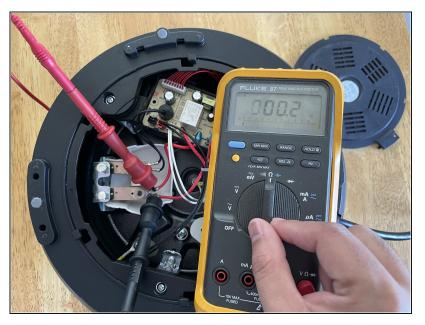
Use a multimeter to test the sensors for proper operation before you reassemble your Instant Pot.
