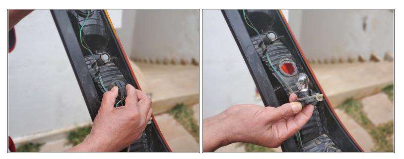
• Remove the bulb socket by making a <sup>1</sup>/<sub>4</sub> counterclockwise twist.
