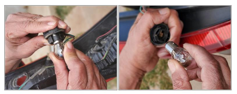
• Remove the bulb from its socket by making a <sup>1</sup>/<sub>4</sub> counterclockwise twist.
