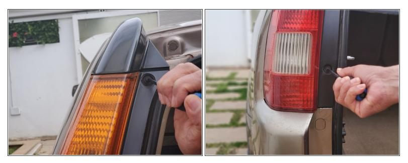
• Remove both screws using the Phillips screwdriver.
