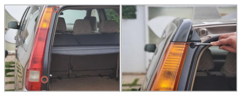
• Remove the tab covering the screws using the flat-head screwdriver.
