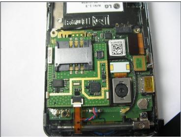
Remove the plastic case to reveal the motherboard.
