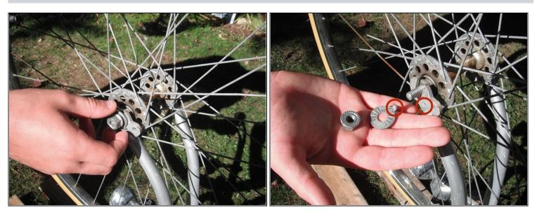
• After removing the nut, also remove the washer under it.
