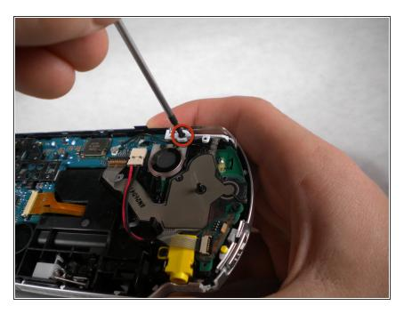
Remove the screw securing the 'R' trigger.
