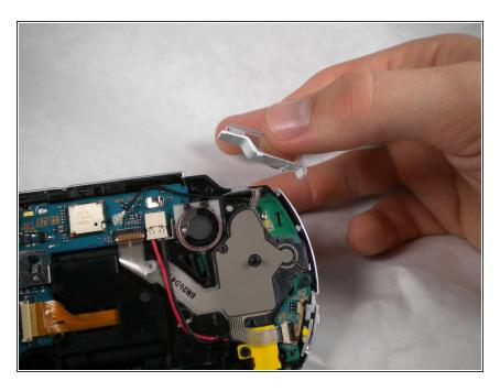
Remove the 'R' trigger from the PSP.
