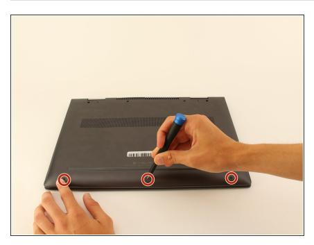
Use a Torx T5 screwdriver (T5 bit) to remove the three 5mm screws near the bottom edge of the laptop.
