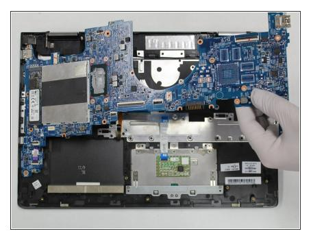
Gently lift the motherboard up and out of the chassis.
