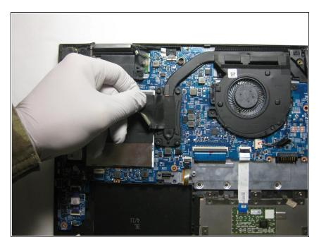
Peel off the tape securing the heatsink.
