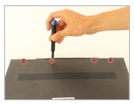
Use a Phillips #1 screwdriver (PH1 bit) to remove the four 6.5mm screws that were underneath the rubber strip.
