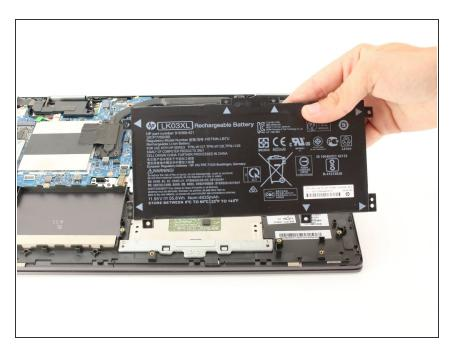
Pull the battery from the connecting port and lift to remove it from the laptop.
