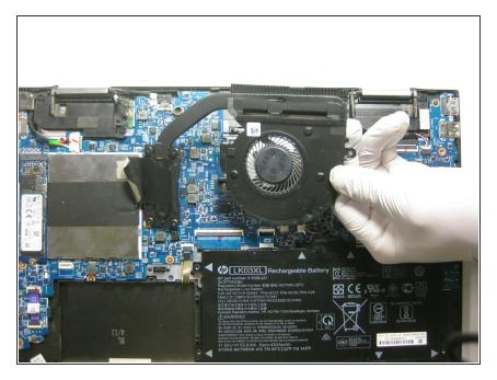
Lift the fan up and off the motherboard.
