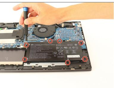
Use a Phillips #1 screwdriver (PH1) to remove the seven 4mm screws indicated by the gray arrows on the battery.
