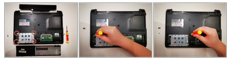
• Remove the four screws from the hard drive support arm using a Phillips #0 screwdriver.
