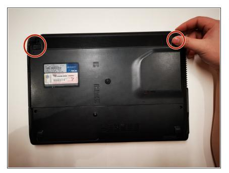
Slide the latch on the right side of the battery on the back of the laptop to the right to the unlocked position.
