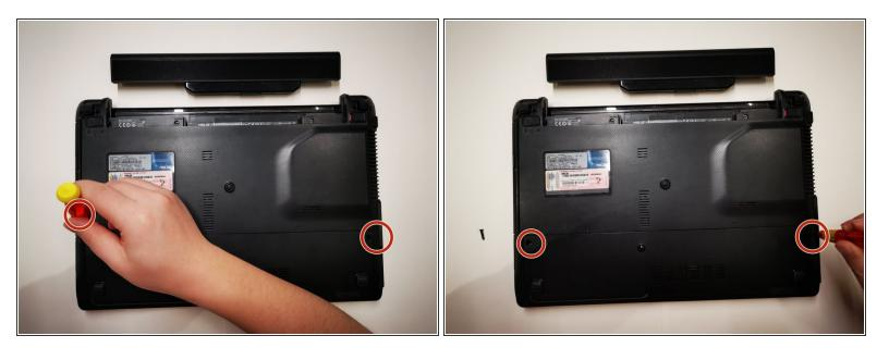
• Remove the two screws on the bottom of the laptop using a Phillips #0 screwdriver.
