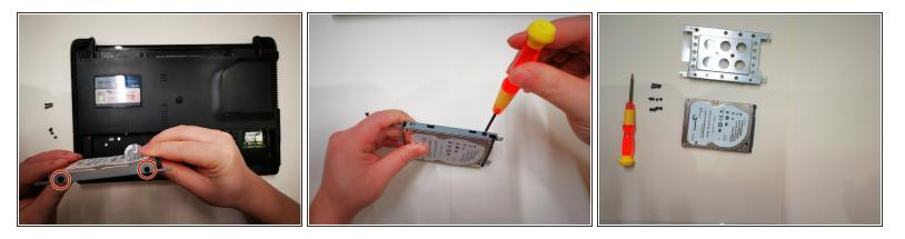
• Remove the four screws on the side of the hard disk support using a Phillips #0 screwdriver.
