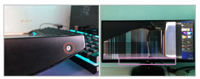
• There are 2 Phillips #2 screws holding the lower trim, with the LG logo, onto the monitor.
