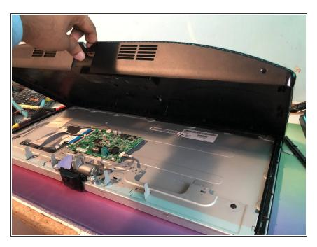
The rear cover separates from the LCD panel, revealing the surprisingly tiny control board
