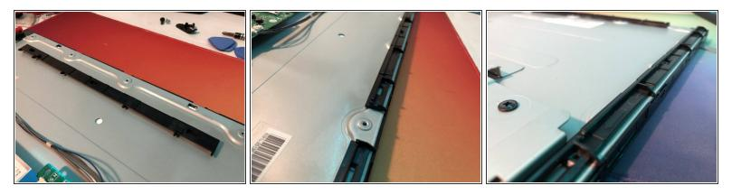
A closer look at the mounting method shows that there are a series of plastic "rods" that slide into slots on the LCD panel frame. The "rods" then attach to the clips on the rear housing as seen in Step 8.
