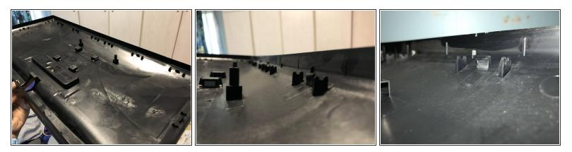
• Some close-ups of the clips and mechanism used to secure the rear cover to the LCD panel
