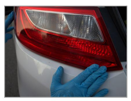
Push the replacement tail light assembly into its original position until it clicks.
