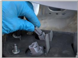
• Plug the four connectors into their corresponding ports of the replacement tail light assembly.
