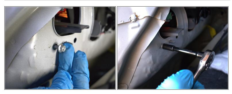
• Tighten the 8mm nuts that were removed during Step 3 using the 8mm socket wrench.
