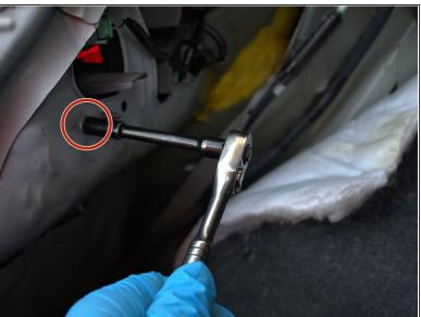
Remove the four 8mm bolts using the socket wrench.
