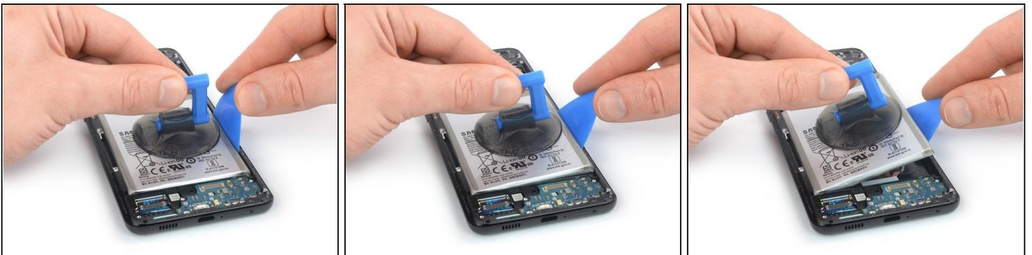
⚠ Take care not to puncture or bend the battery during the removal procedure—a punctured or bent battery may leak dangerous chemicals or cause a thermal event. In case you're struggling to pull up the battery apply more isopropyl alcohol and try again.
