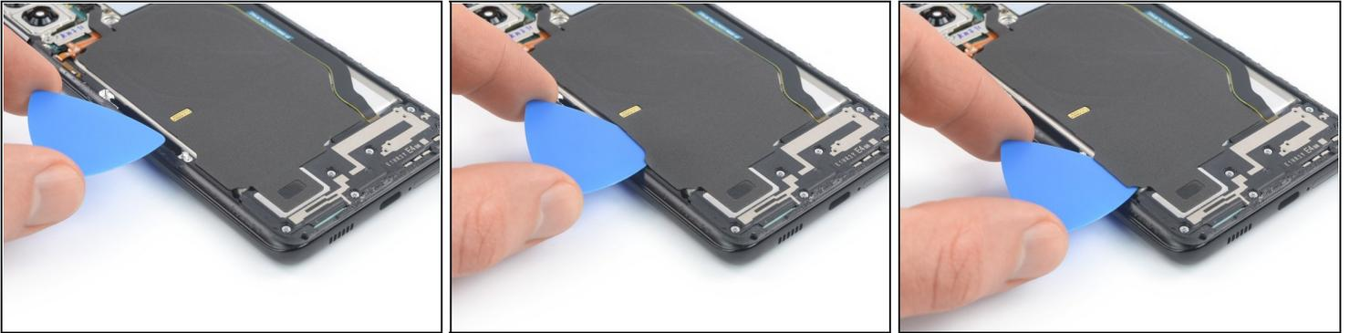
⚠ Take care not to puncture or bend the battery with your tool—a punctured or bent battery may leak dangerous chemicals or cause a thermal event.
