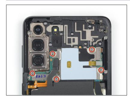
Use a Phillips screwdriver to remove the five 3.9 mm-long screws securing the NFC antenna and charging coil assembly.
