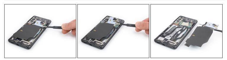
• Use a pair of tweezers or your fingers to carefully remove the NFC antenna and charging coil assembly.
